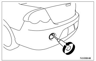
1. Remove the light mounting screw and pull the entire light bracket out.  $\,$
